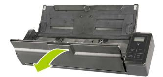
**3.** Wipe the separation pad, rollers and the glass with the included cleaning cloth.
