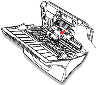
5. Insert and guide the left end of new Separation Roller in its hole, then push the right end down into the U-shaped holder.
