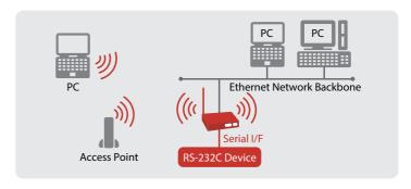
eCable Mode: Serial data can be tunneled over the network between devices connected to SD-320AN.
