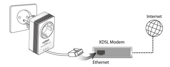
2. Connect another powerline adapter to your computer, and then plug it into a power socket.
