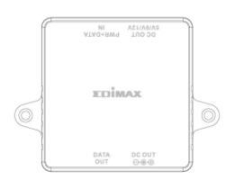
**DATA OUT**: Connect to the Ethernet device with CAT5 UTP cable to transmit data.
